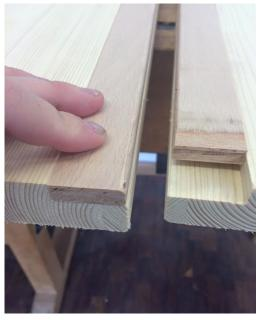
**STEP 4:** Cut wood top pieces and take long edges off for textile installation. Cut new wood pieces to fill in long edges, since blade removes too much material. Sand edge pieces to deal with textile thickness. Then drill and sink screw holes for textile installation.
