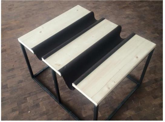
**STEP 6:** Cut textile into desired length and size. Then install and drill the textiles onto the frame. Finish / Stain wood top surface. Enjoy your table!
