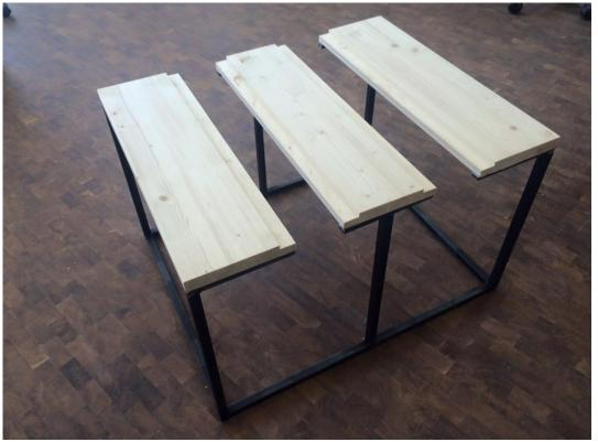
**STEP 5:** Clean and shine steel with suggested cleaning products. Once cleaned and dry, add wood top pieces to frame. Check that edges and screw holes are aligned.
