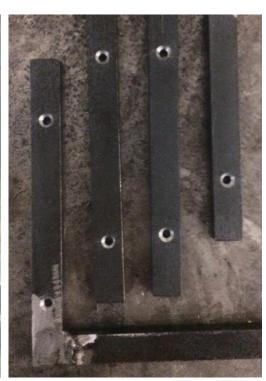
**STEP 2:** After bottom frame pieces are welded and are square, cut top steel bars to size. Then drill screw holes in pieces that will be used later to attach wood tops to table.
