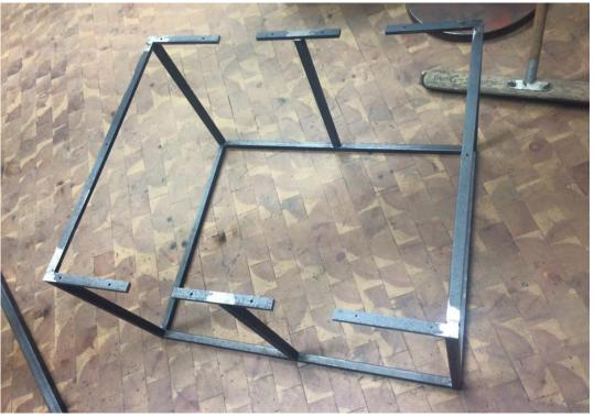
**STEP 3:** Weld steel bar pieces to the completed frame. Make sure the pieces are flat and squared so the wood top surface of the table is flat and square to the ground.
