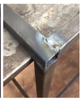
**STEP 1:** Cut steel into 4 sizes, 10 pieces in total. While keeping edges square weld pieces together into frame.
